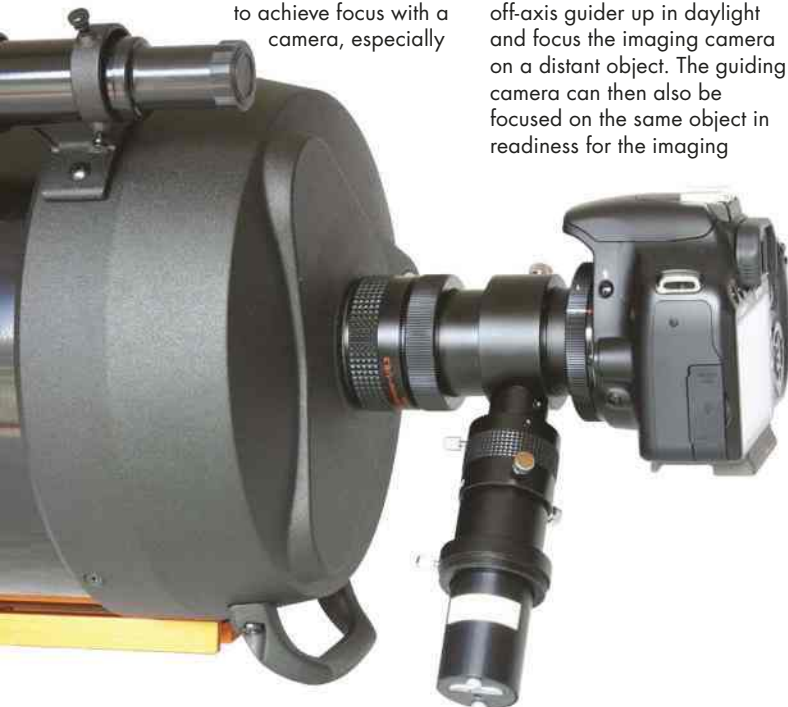
▲ An off-axis guider and camera sit between the main imaging camera and a scope’s eyepiece holder
